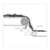
SR separators are typically used as head pulleys in belt conveyors. As tramp metal nears the separator's magnetic field, it is attracted and held to the conveyor's belt until it reaches the underside of the conveyor, where it passes out of the magnetic field and discharges into a chute or bin. The cleaned, contaminant-free material discharges from the top of the conveyor, away from the tramp metal.
