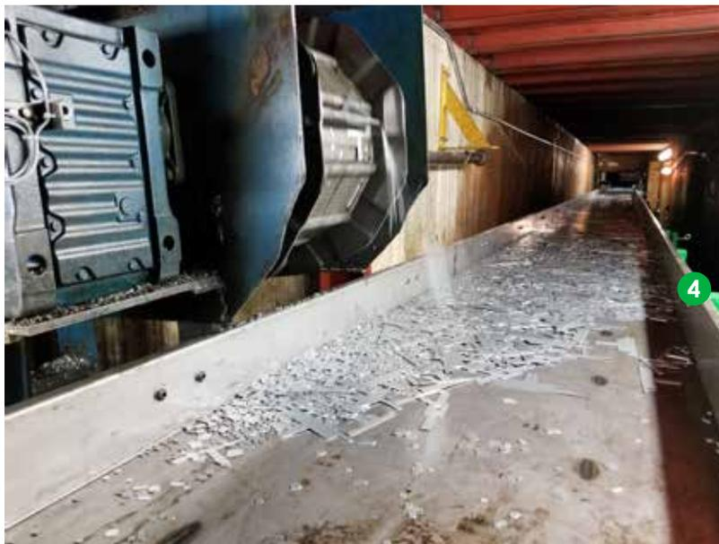
MPI's M-10000 Series High-Capacity Floor Mounted Electric Shaker Conveyor is designed to transfer scrap metal, bulk products, or bulk materials reliably over long horizontal distances. The horizontal motion conveyor is designed to transfer at rates of over 10,000 pounds per hour and distances of hundreds of feet. The shaker conveyor features a formed steel pan that is driven by a single drive at a smooth, low frequency to convey materials in a horizontal motion.
