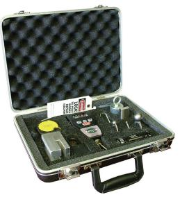
NIST-certified scales should be used by your magnetic separator auditor and made available to food processors as part of a kit to conduct their own pull tests.
