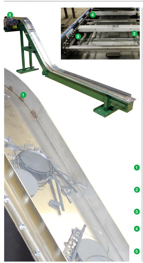
Rugged, reliable and robust, MPI's Beltless Magnetic Conveyors efficiently move ferrous metal, stampings, turnings, chips, fasteners, scrap and more, wherever it needs to go. Powerful permanent magnets, located below a nonmagnetic stainless steel slider bed, transport parts without fail and without downtime, even when faced with the most challenging applications. As the magnets move, objects travel along the conveyor and into a bin for easy removal or transport.
