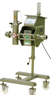
Cassel's "IN MEAT" compact Metal Detector is designed for sausage stuffers and is easily transportable via its wheeled-base. An integrated gas spring provides for quick height adjustment (33.5" - 47.2"), allowing installation between the stuffer and clip machines. Links and adapters are available for nearly every type of stuffer and clip machine. A variety of reject systems are offered.
