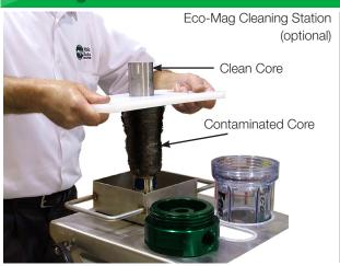
Using the supplied cleaning tool, a fully contaminated core can be cleaned in under 30 seconds, leaving you with only metallic particles, which can be easily disposed of, no dirty cartridges.
