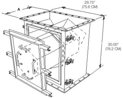
NOTE: FFC SERIES MAGNETS ARE SUPPLIED WITH 2" FLANGES. INTERIOR HOUSING WIDTH = 25.5" (64.8 CM)
