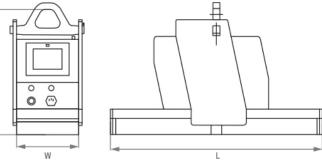
Universal large steel lifting eye with safety bail sensor makes it impossible to disengage magnet during lifting
