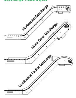
**BLM Series:** MPI offers three series of magnetic conveyors. Each larger series has a larger body to accommodate larger magnetic cartridges and heavier duty internal chain designed to handle more difficult scrap or higher scrap rate capacities. MPI will help you select the correct duty for your application.
