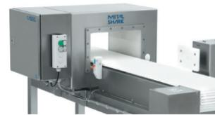
As raw materials arrive in the processing area, they must be examined for metal contaminants (5 -10 mm) such as knife blades, metal gloves, meat etc. Typically, a metal detection system comprised of a conveyor-style metal detector with an upgraded HW conveyor, and LPW or HPW option would be selected. The HW conveyor features an open stainless frame without dirt traps, a waterproof stainless drum motor, fully encapsulated sensor head and an FDA/USDA-approved transfer belt.
