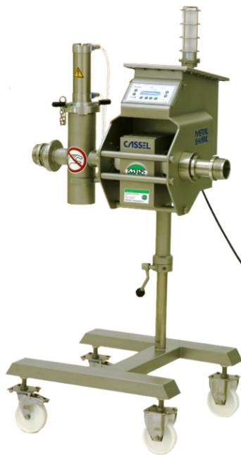
Cassel's "IN MEAT" compact Metal Detector is designed for sausage stuffers and is easily transportable via its wheeled-base. An integrated gas spring provides for quick height adjustment (33.5" - 47.2"), allowing installation between the stuffer and clip machines. Links and adapters are available for nearly every type of stuffer and clip machine. A variety of reject systems are offered.
